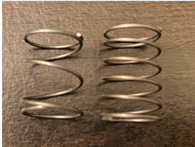
Figure 17: Two different kinds of springs from the motor shaft assembly
